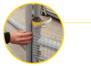
Install the Snake Guards on each adjacent Fence Panel. By hand, separate the two tubes of the Snake Guard and slide the guard down to the base of the stand keeping the spring nut on the inside of the fence and the black caps on top. Re-close the metal strap loop connecting the panels.
